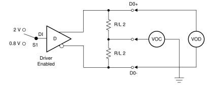
Figure 7-1. Differential Driver DC Test Circuit
