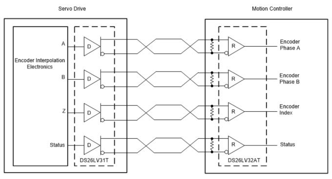
Figure 9-1. Application Schematic - Encoder Application
