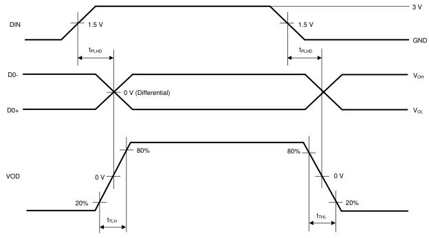
A. Generator waveform for all tests unless otherwise specified: f = 1 MHz, Duty Cycle = 50%  $Z_O$  = 50  $\Omega$ ,  $t_r \le 10$  ns,  $t_f \le 10$ .
