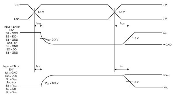
Figure 7-5. Driver Single-Ended TRI-STATE Waveforms
