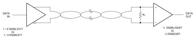
Figure 9-2. Typical Driver Connection - R<sub>T</sub> is optional although highly recommended to reduce reflection
