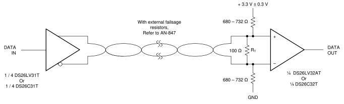
Figure 9-3. Typical Driver Connection
