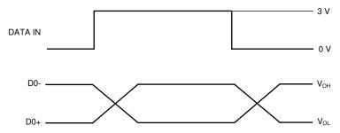
Figure 9-4. Typical Driver Output Waveforms
